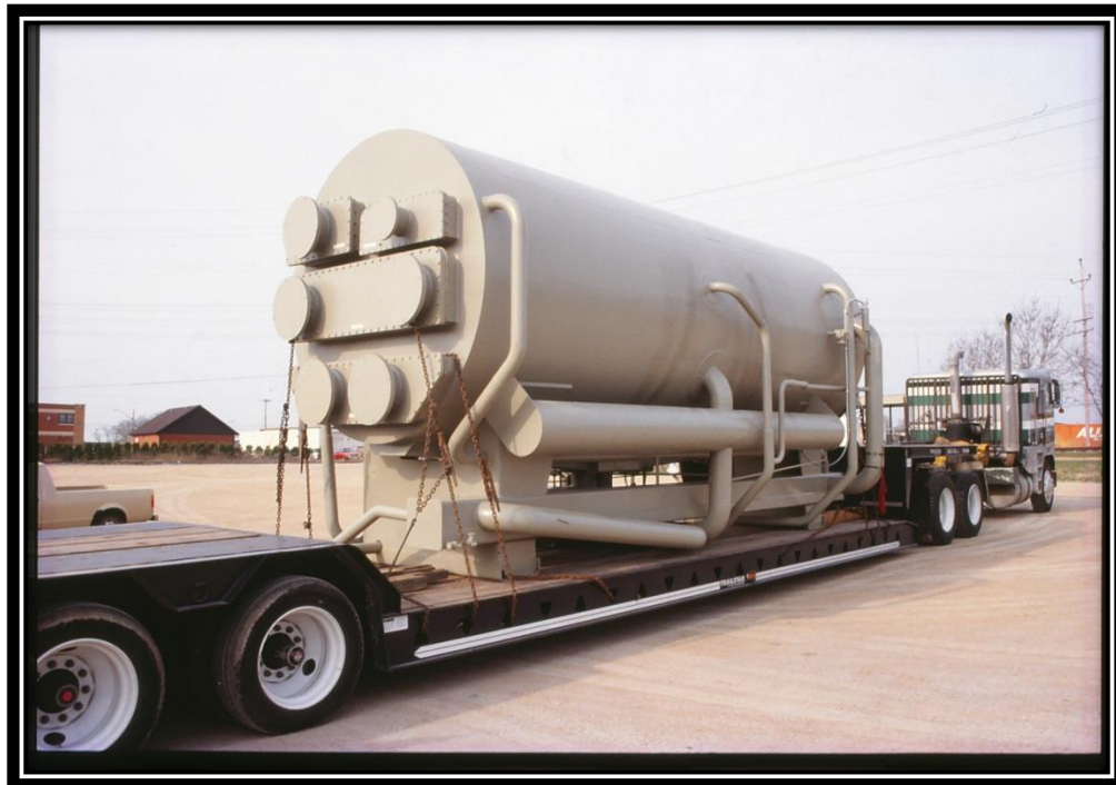
Figure 6. Absorption unit shipping to job site
