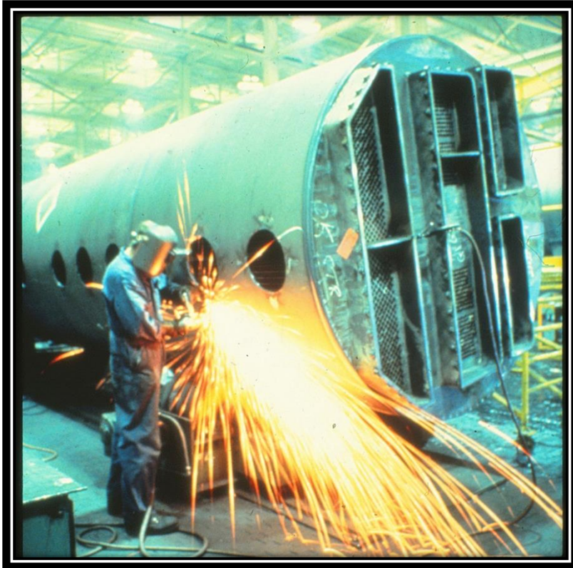
Figure 5. Factory worker welding vessel
